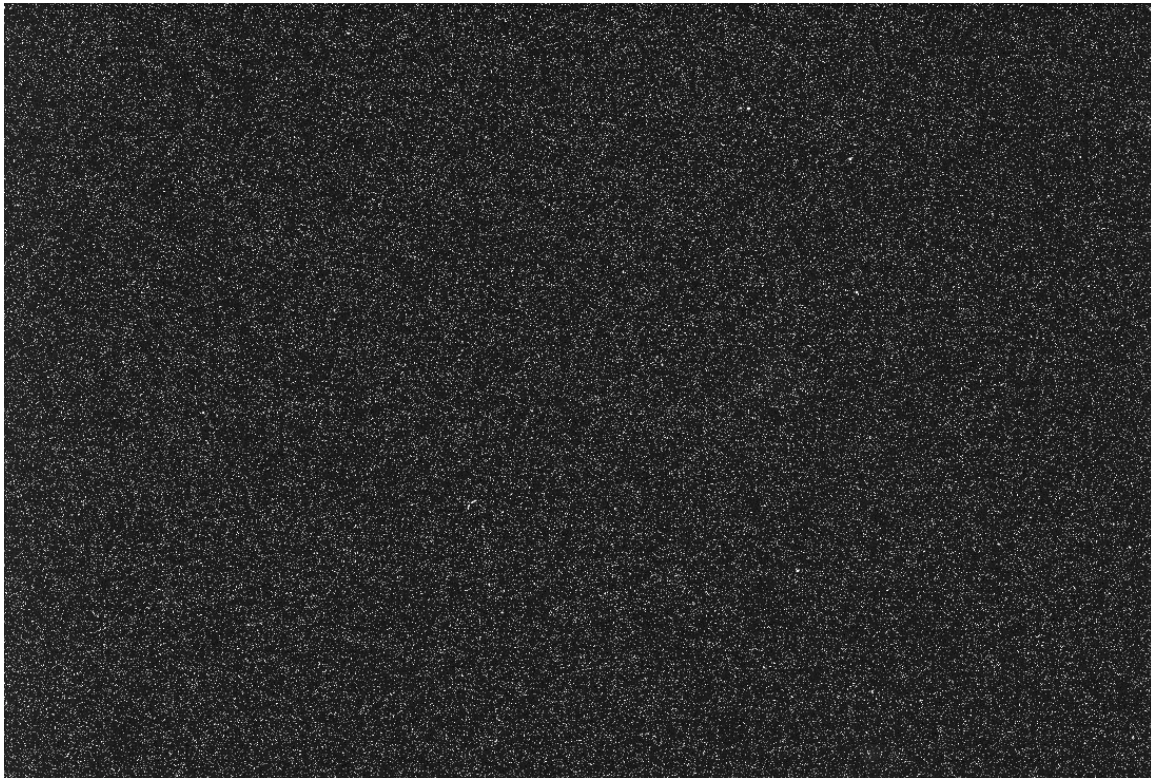
Figure 25 - A dark frame records the dark current of the CCD chip.
