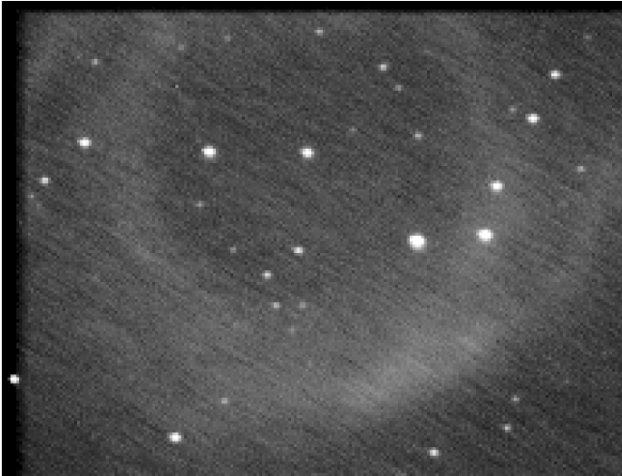
Figure 39 - A Track and Accumulate image showing correlated noise from too short of an exposure time for the individual images.
