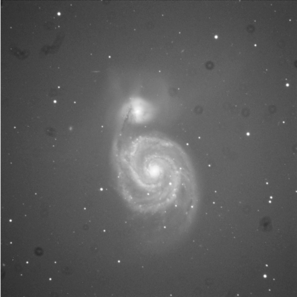
Figure 26 - An image showing vignetting (darkening away from the center) and shadows from dust on optical surfaces.
