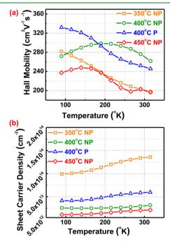
**Figure 6.** (a) Hall mobility and (b) sheet carrier density as a function of temperature in Ge layers grown at 350, 400, and 450 °C, respectively. Ge layers were grown with without pause (NP) and with a long growth pause (P).
