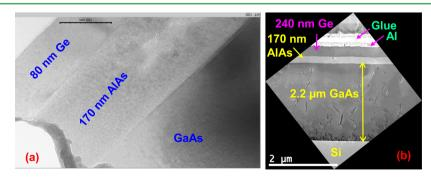
Figure 5. (a) Cross-sectional TEM micrograph of 80 nm Ge grown on GaAs substrate using a 170 nm AlAs buffer layer. The granular spots in some areas of AlAs layer are due to the damage during ion milling process. (b) Cross-sectional TEM micrograph of the Ge/AlAs/GaAs/Si structure. The TEM measurement was performed after depositing the aluminum metal.
