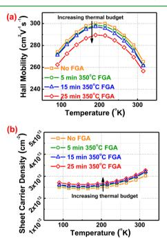
Figure 7. (a) Hall mobility and (b) sheet carrier density as a function of temperatures in Ge layers grown at 400  $^{\circ}$ C without long growth pause under different forming gas annealing (FGA) time at fixed annealing temperature of 350  $^{\circ}$ C, respectively.
