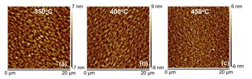
Figure 3. Surface morphology of the epitaxial Ge layers grown at three different growth temperatures on  $(100)/2^{\circ}$  GaAs substrates. The measured surface roughness are in the range of 1.8-2.5 nm.
