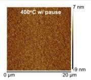
**Figure 4.** Surface morphology of the epitaxial Ge layer on  $(100)/2^{\circ}$  GaAs substrate grown at 400 °C with 12 h growth pause after the AlAs layer growth. The measured surface roughness was 2.21 nm.
