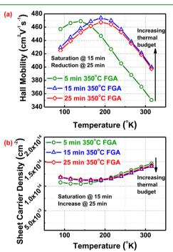
**Figure 8.** (a) Mobility and (b) sheet carrier density as a function of temperature in the Ge layer grown at 400 °C under different forming gas annealing FGA time, respectively, on Si using a composite AlAs/GaAs buffer layer.
