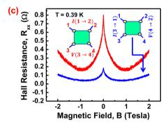
**Figure 9.** (a) Antisymmetric component of the Hall resistance,  $R_{XY}$  as a function of magnetic field over  $\pm 9T$ , with the very linear dependence on magnetic field demonstrating single carrier behavior. (b) Symmetric component of the Hall resistance,  $R_{XX}$  as a function of magnetic field over  $\pm 9T$ . (c) High-resolution traces, with different resistance offsets subtracted, emphasizing the weak-localization behavior at low magnetic fields.
