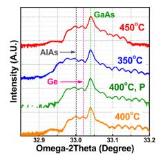
**Figure 2.** X-ray rocking curves for the 80 nm Ge layer grown on  $(100)/2^{\circ}$  GaAs substrates at 350, 400, and 450  $^{\circ}$ C, respectively. The Pendellösung oscillations from these samples show the superior epitaxial crystalline quality. The X-ray curves were shifted vertically for clarity. The "P" represents the long growth pause prior to Ge layer growth.
