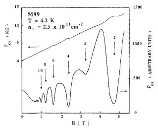
FIG. 3. Transport coefficients  $\rho_{xx}$  and  $\rho_{xy}$  for sample M99 are shown as a function of magnetic field at a fixed gate voltage. The vertical arrows indicate some of the Landau-level filling factors at which the integral quantum Hall effect is observed.
