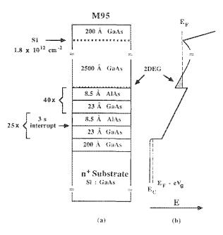
FIG. 1. Schematic description of an ISIS structure. Shown on the right is the potential diagram corresponding to the accumulation mode, achieved by applying a positive gate voltage  $V_g$  to the  $n^+$  substrate. On the left, the design structure for sample M95 is schematically shown. Note the use of a thin-layer GaAs/AlAs superlattice in place of AlGaAs barrier.
