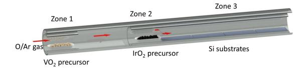
**Figure S1.** A schematic of the three-zone quartz tube furnace used to grow  $Ir_{1-x}V_xO_2$  nanowires.
