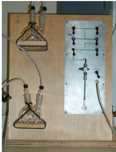
Figure 4.12: Prototype source loading station to create ^{222}\text{Rn} sources.
