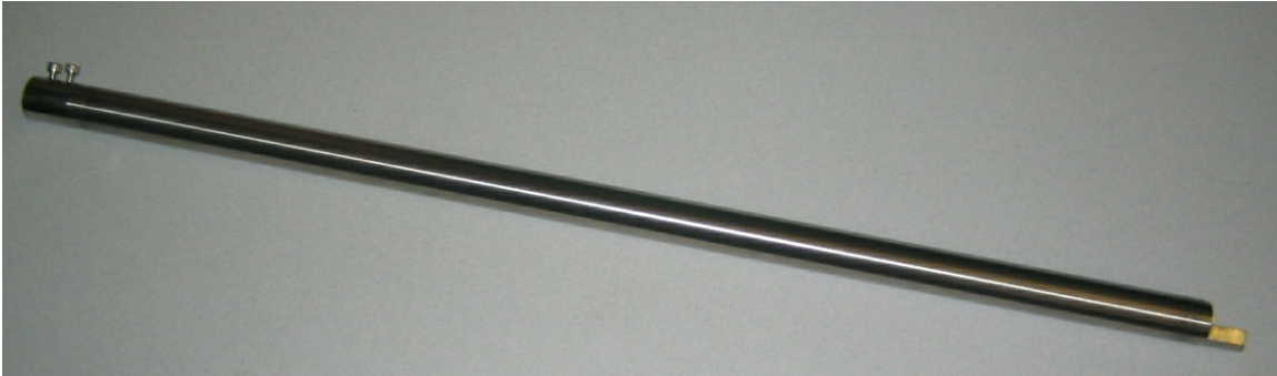
Figure 5.3: Source insertion rod with couplers welded on. Insertion rods are completely independent from each other so that they do not need to be connected in a particular order.
