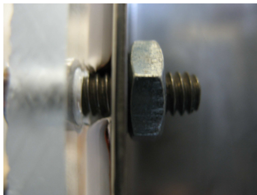
Figure 4: Sample 3 Exterior View, Note that the seal has ripped around bolts
