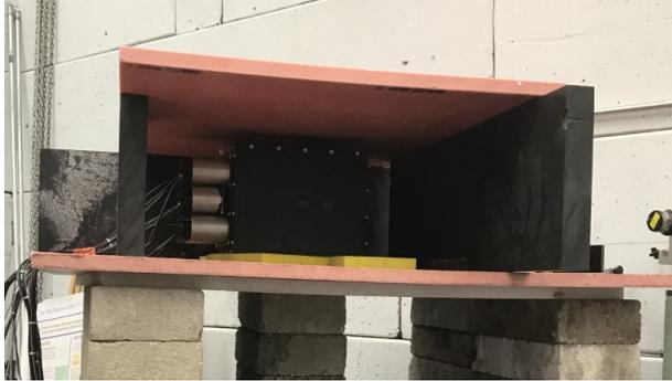
Figure 2. MicroCHANDLER placed within an enclosure of borated polyethylene. The pink sheets contain a 5% concentration of Boron 10 while the black sheets contain 30%.
