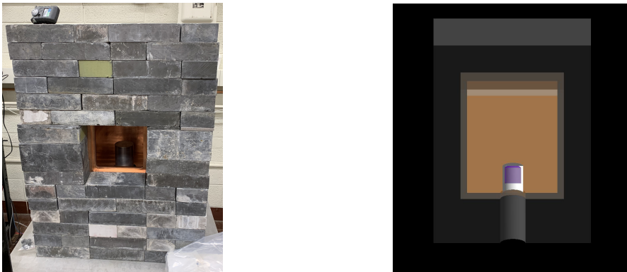
Figure 1: Left: The "MELISSA" Canberra LB coaxial HPGe detector in a copper and lead shield. Right: A Monte Carlo simulation of the empty detector in Geant4.
