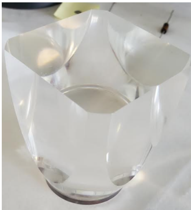
Figure 3: The new light guides planned for use in miniCHANDLER.
