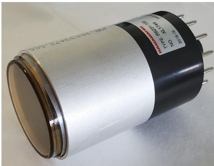
Figure 4: A picture of a Hamamatsu R6231-100 PMT.
