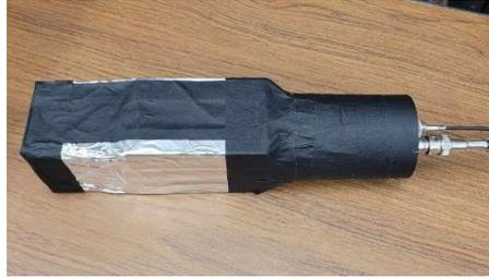
Figure 4: A detector made of a scintillator, collimator, and a PMT
