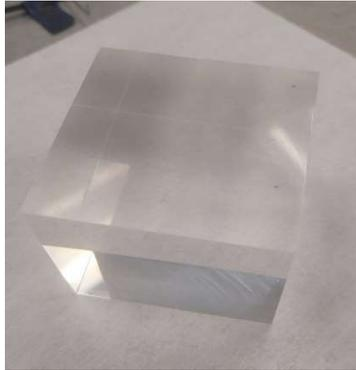
Figure 1: A plastic scintillator cube
