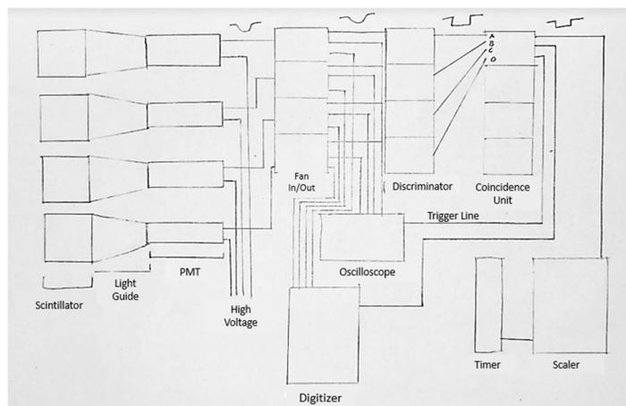
Figure 3: Signal logic to allow single and up to four-fold coincidence detection
