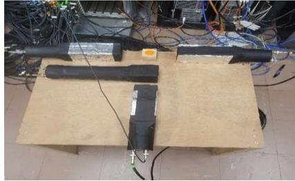
Figure 5: Quadruple coincidence setup for  $0^\circ$
