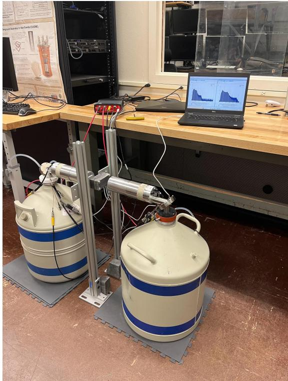
Fig 1: HPGe Detectors VTGe3 (left) and VTGe4 (right) set-up connected to CAEN DT5780 DAQ module facing a sample of  $\text{Na}^{22}$  suspended in a lead collimator.
