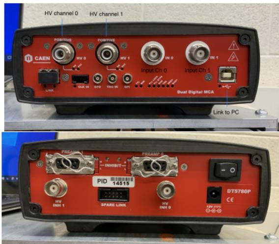
Fig 3: (Top) Front inputs for CAEN DT5780P DAQ for HV, Input, and USB. (Bottom) Back of DAQ unit displaying inputs for Inhibitor and Preamp. [3]
