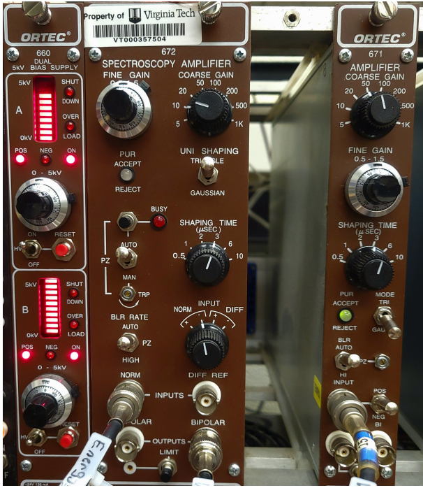
FIG. 12. An image of the 5-kV radiation detector bias supply (left), Model 672 spectroscopy amplifier (middle), and Model 671 spectroscopy amplifier (right)
