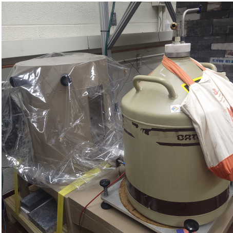
FIG. 7. Outside of VT1. The dewar is located on the right with the detector chamber in its shielding connected to the left
