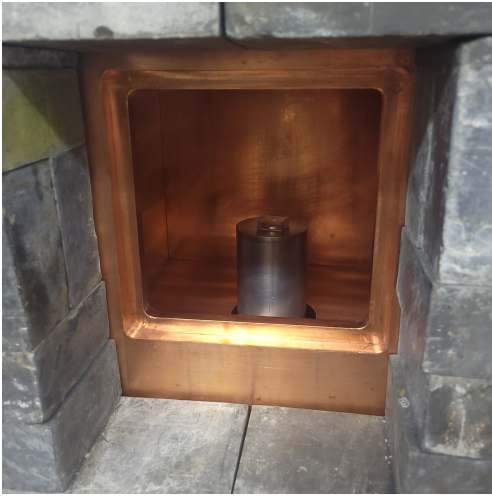
FIG. 11. Inside of VT2. Here we can see the detector chamber and a radioactive collaboration placed inside.
