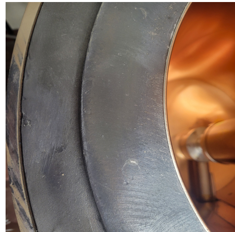
FIG. 5. This image shows the thick lead shielding around the copper barrier that surrounds VT1's detector element.
