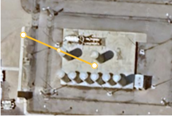
FIG. 2. Detector placed outside outer perimeter fence to center of storage.
