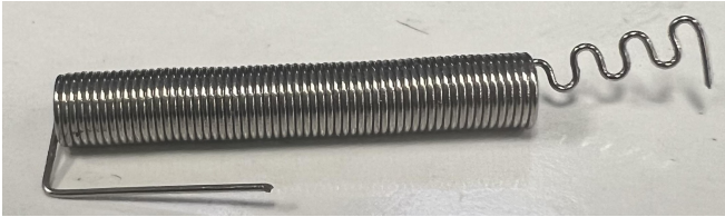
FIG. 3. Spring-tempered 304 Stainless Steel Spring used in DS-20k; notice the 66 coils, square hook, and switchback hook coils for wire attachment.
