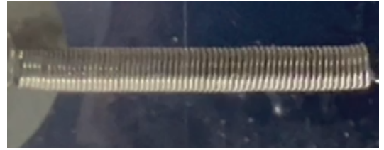
FIG. 6. A demonstration of nonuniform pretension in a spring; a specifically chosen mass is hung from the spring such that it has enough weight to overcome the pretension of the lower half of the spring but not the upper half - as seen in the prevalence of gaps between coils in the lower but not upper half.
