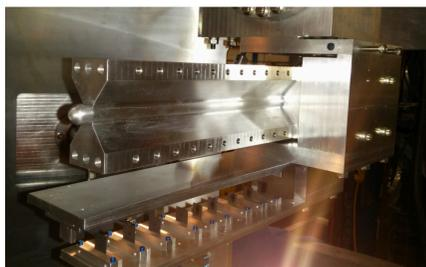
The experiment took place in Hall A of Jefferson Lab. The incident electrons came from JLab's CEBAF beam. The beam struck either a solid titanium foil target or gaseous argon closed cell (shown above). The final state electrons and protons were separated into the left and right high-resolution spectrometers, respectively. These detectors measured several kinematical variables, including the missing energy and momentum of the final state nucleus.
