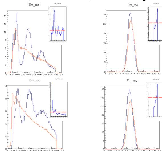
The plots above show the missing energy for argon (top left), missing momentum for argon (top right), missing energy for titanium (bottom left), and missing momentum for titanium (bottom right). The data with background subtracted is orange, the MC is black, and the inset shows the data-to-MC ratio distribution. We also scaled the data using the total charge detected and the efficiency (good events per event that occurred) of the detector.
