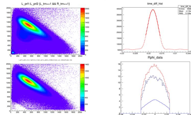
The top right plot above shows the distribution of time between the event being detected in the left and right spectrometer. We used the background on either side of the peak to find the distributions of background events. The lower right plot above has distributions of the out-of-plane angle in the proton arm with the data in red, the MC in black, and the background in blue.
