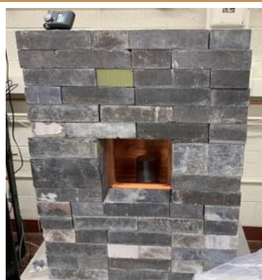
The "MELISSA" Canberra LB high purity germanium detector inside a copper housing and lead brick shield.
