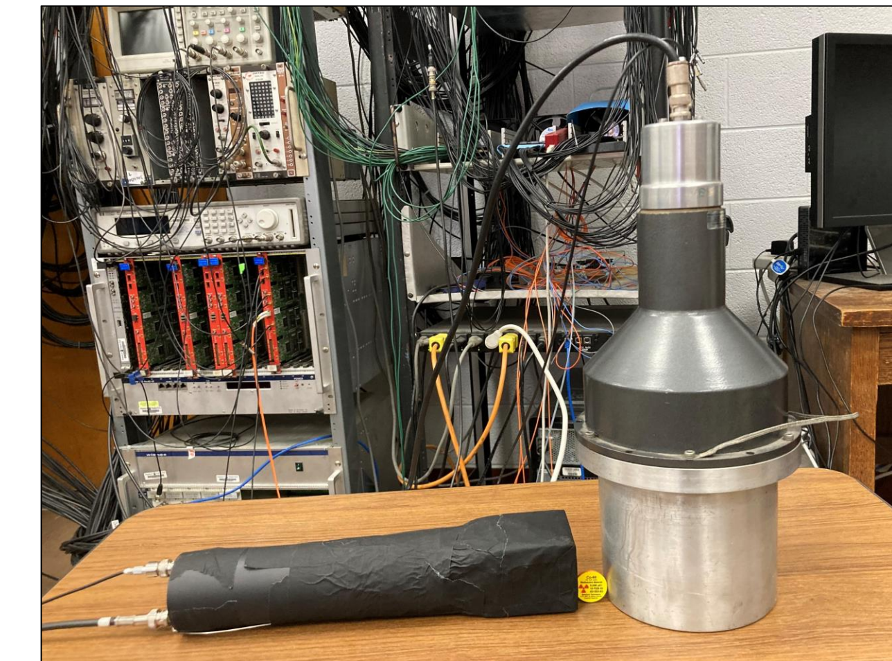
FIG. 1. The PVT detector is shown on the left, covered with paper to avoid external light. A sample of Co60 is between the PVT and the NaI(Tl) detector on the right.
